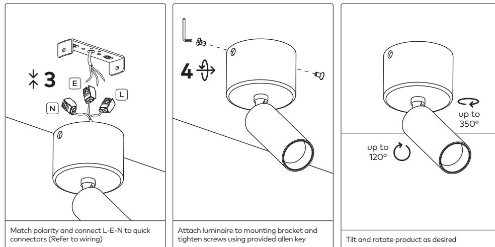
Match polarity and connect L-E-N to quick connectors (Refer to wiring)
