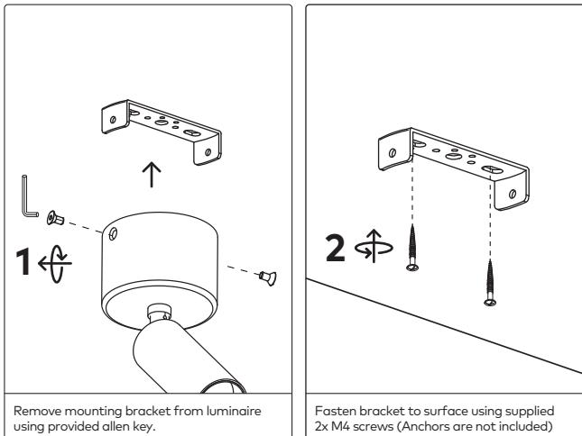
Remove mounting bracket from luminaire using provided allen key.
