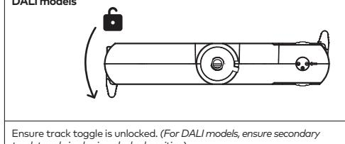
Ensure track toggle is unlocked. (For DALI models, ensure secondary track toggle is also in unlocked position)
